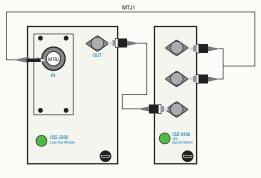
Basic configuration for testing multifiber connectors such as MTP and MT-RJ.
